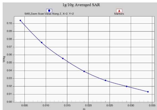
Fig.A.1- 3 Z-Scan at power reference point (PCS1900)
