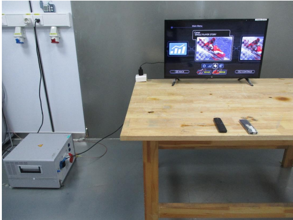
Conducted Disturbance Emissions on AC mains
