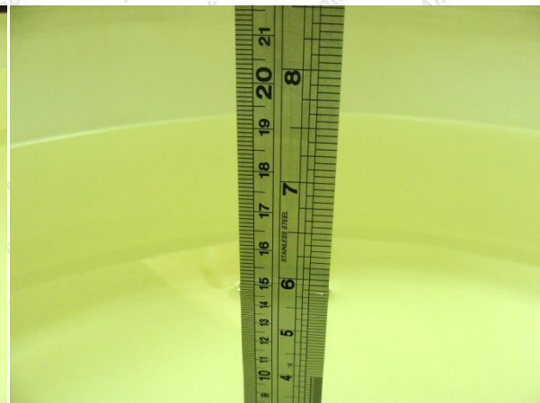
Photo of Liquid Height for Body SAR
