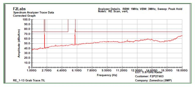
Note: In the above plot, the emissions spikes shown are from the fundamental frequencies of a certified Wi-Fi module.
