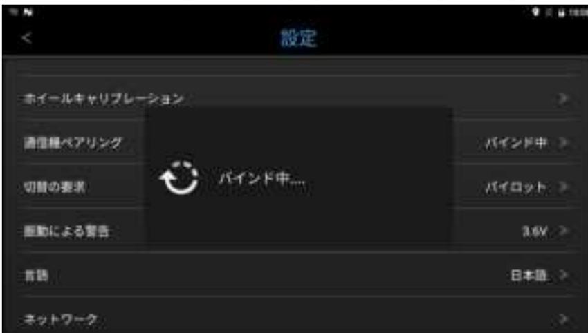
(5) When the pairing is completed successfully, the status of [Pair with communication device] will be displayed as [Binding complete] as shown below.
