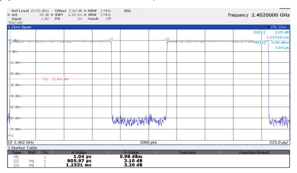
Duty cycle correction according to ANSI C63.10 section 7.5:
