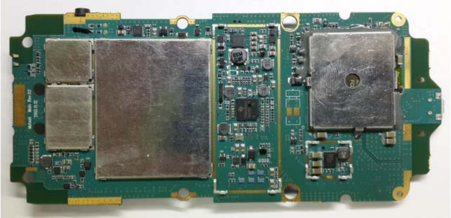
Main PCB Top with shield can
