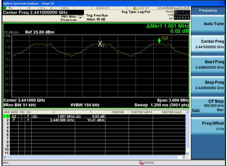
Carrier Frequency Separation (AFH) <u>Hopping mode : Enable & π/4DQPSK</u>
