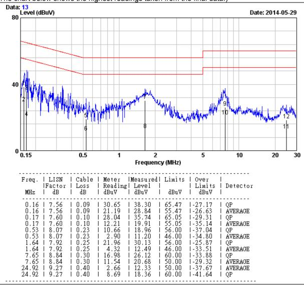
REMARKS : 1. Level (dBuV) = Read Level (dBuV) + LISN Factor (dB) + Cable Loss (dB) 2. Over Limit (dBuV) = Measured Level (dBuV) – Limits (dBuV)
