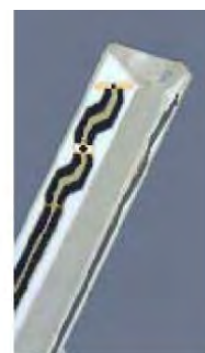
Figure E.2.2 Probe Thick-Film Technique
