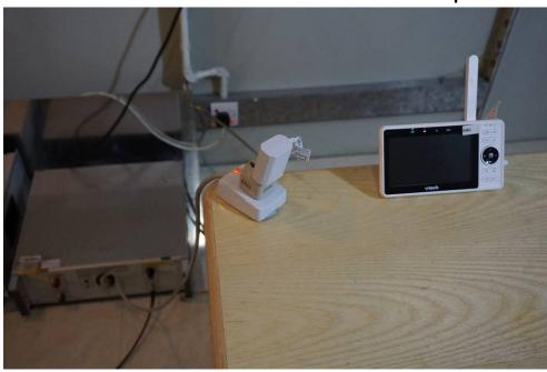
Radiated Emissions (30MHz-1GHz) Test Setup
