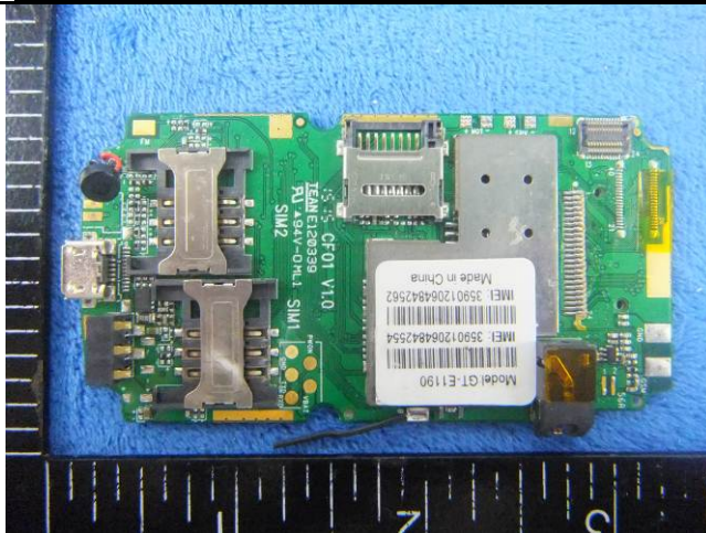
Mainboard With Shielding - Front View
