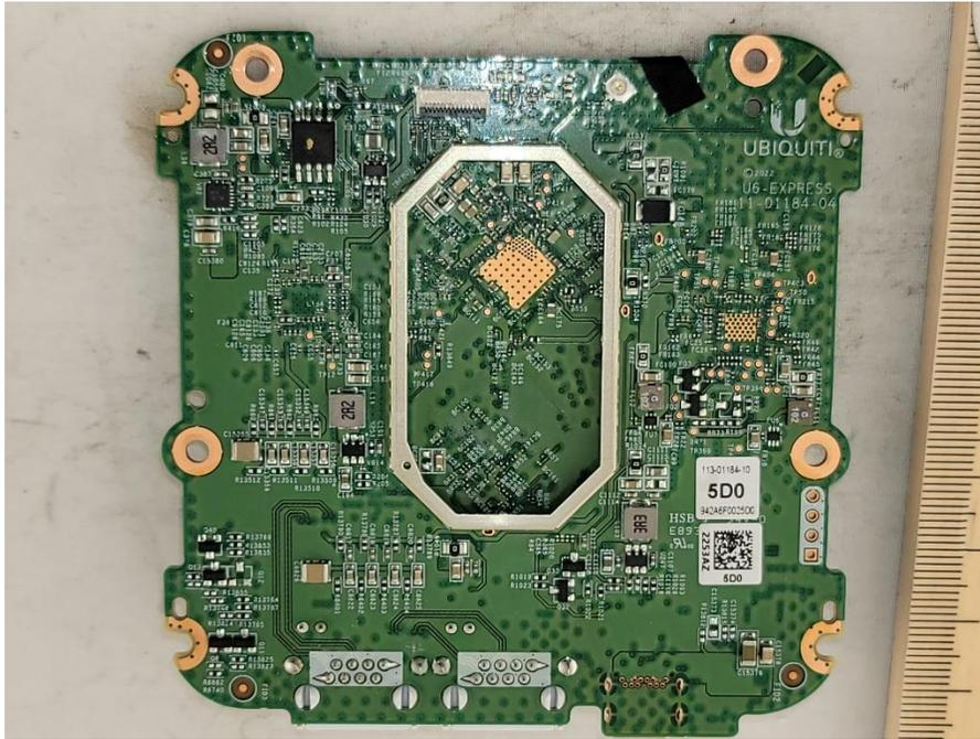
**Photograph 5: PCB EMI Shield Removed**
