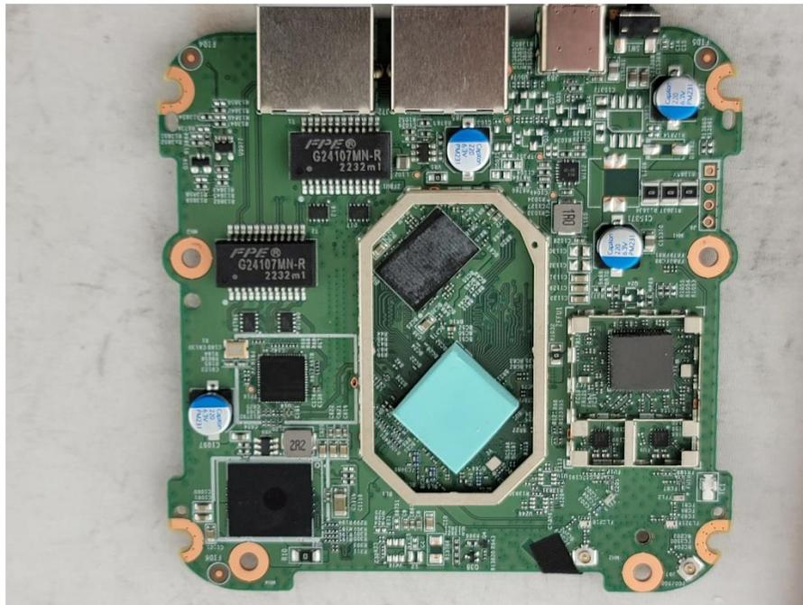
**Photograph 4: PCB EMI Shields removed**
