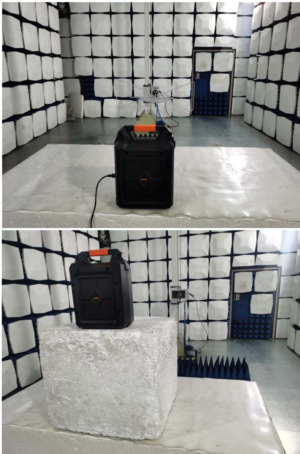
Radiated emission test view
