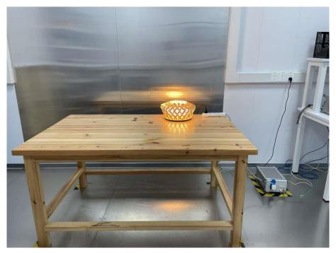
**Radiated Emission Test View 1**
