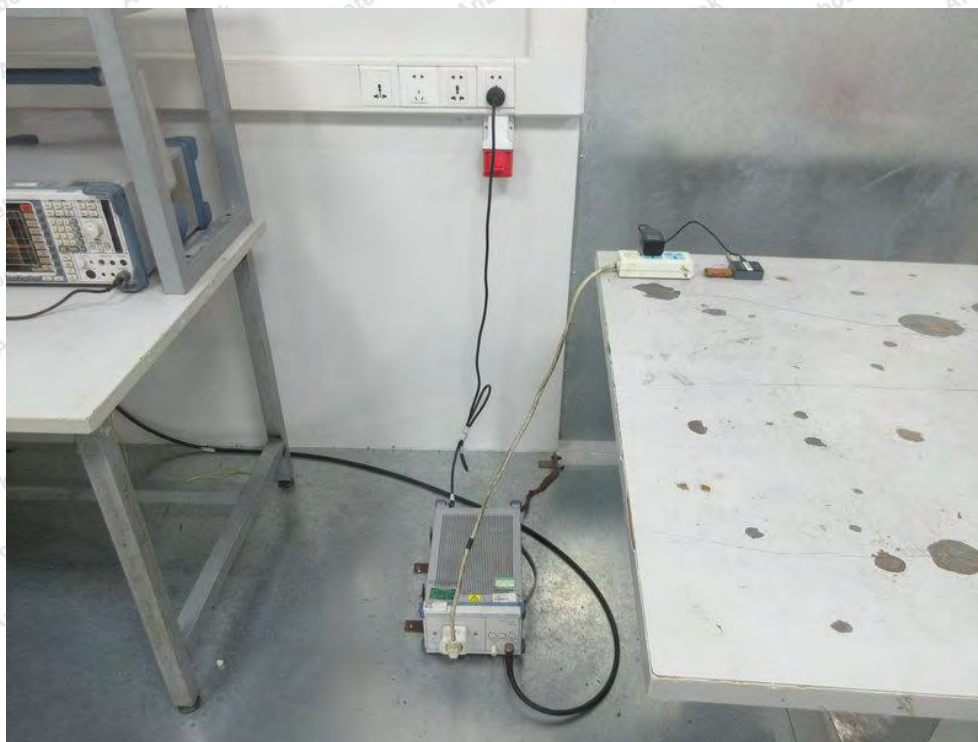
Photo of Power Line Conducted Emission Test
