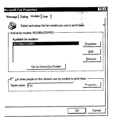
Select "RCV56HCFSPPCI" under "Available Fax modems", click "Set as Active Fax Modem", and then OK. At this point, Microsoft Exchange is configured to use the RCV56HCF/SP. Refer to Microsoft Exchange's on-line help feature to send and receive faxes. When using other TAPI applications, make sure that "RCV56HCF/SP" is the selected modem before attempting connections.
