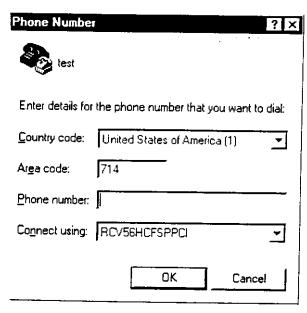
Select "RCV56HCFSPPCI" under "Connect using:", and fill in the other parameters and click OK.
