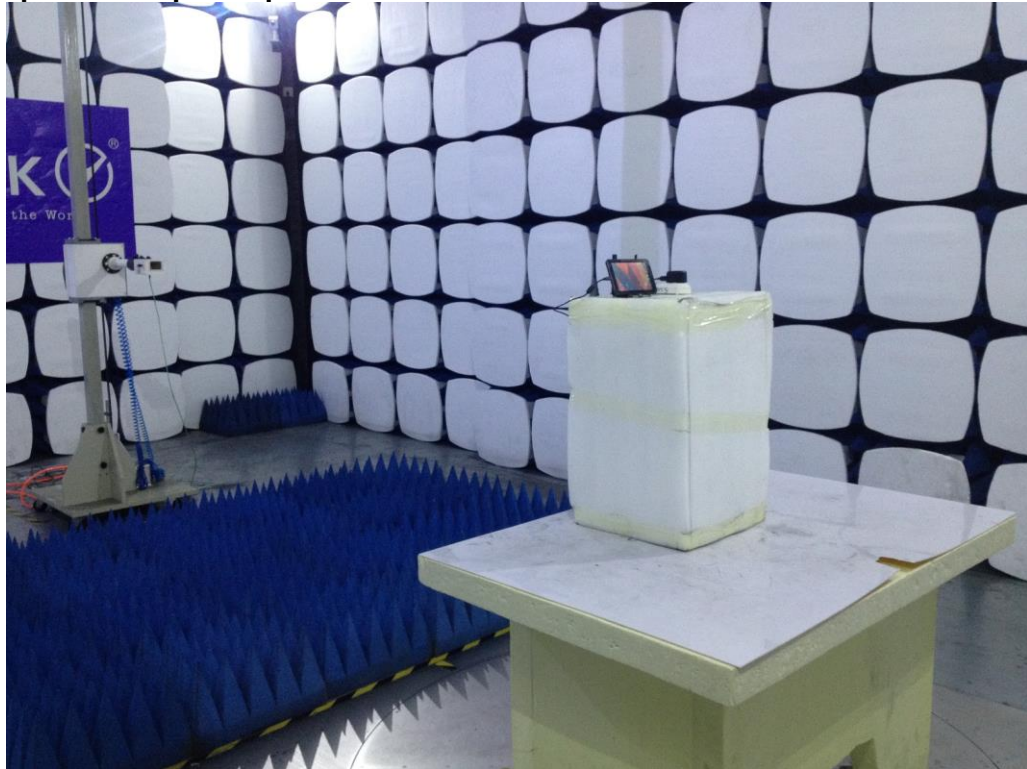
Photograph 5: Set-up for Spurious Emissions for 18 - 40GHz
