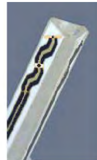
Figure 3.3 Probe Thick-Film Technique
