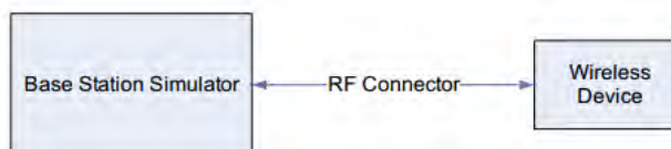
Figure 10.1 Power Measurement Setup
