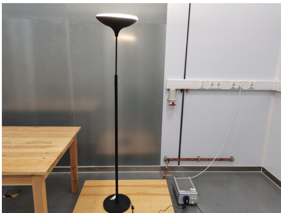
Fig. 4 Power line conducted emission setup photo
