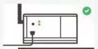
When the device is ready the green LED will be visible. For devices with bluetooth a slow flashing indicates the hotspot is ready for pairing. Press and hold the button for 10 seconds to activate pairing
