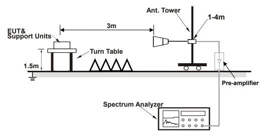
For radiated test above 18GHz
