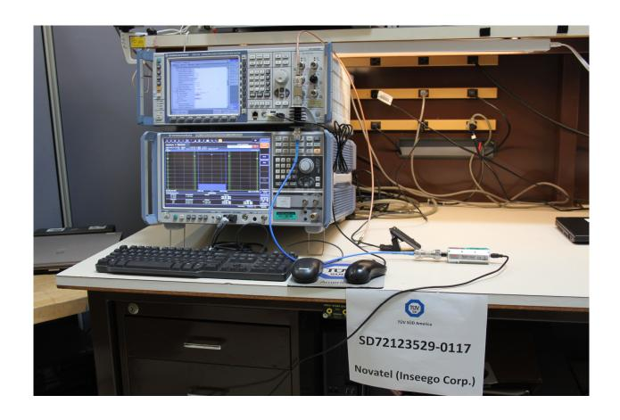
**Conducted Antenna Port Test Setup**
