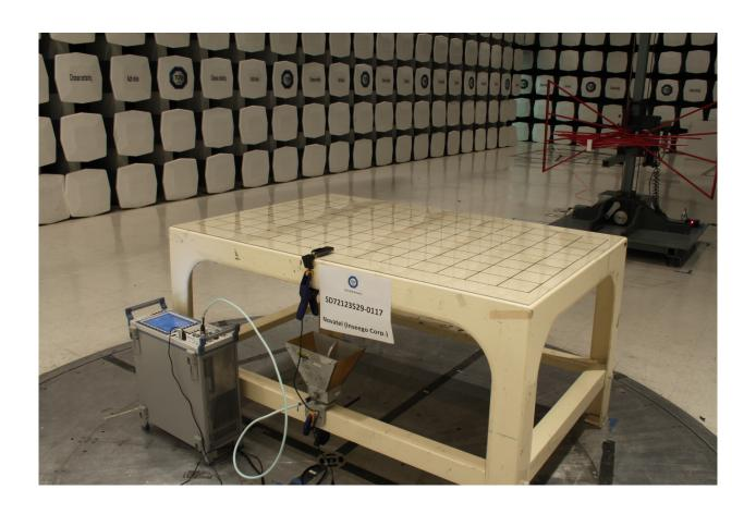
Radiated Emissions Test Setup (below 1GHz)
