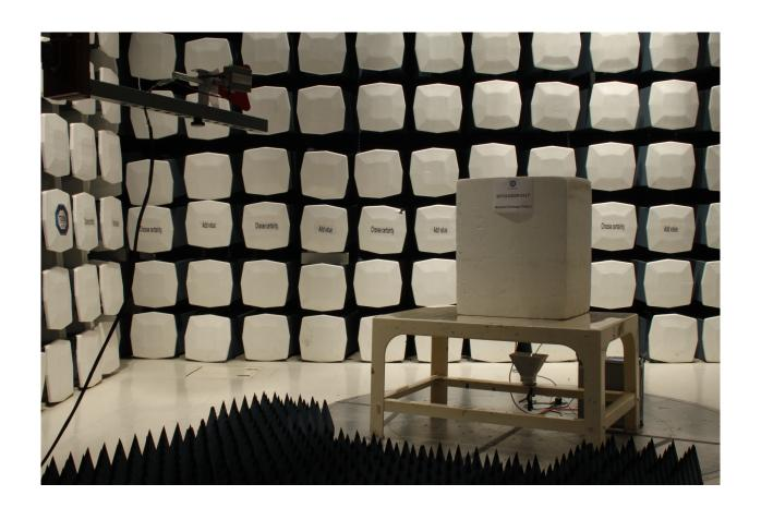
Radiated Emissions Test Setup (above 1GHz)
