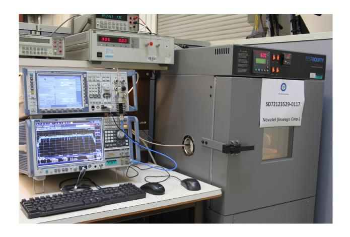
Frequency Stability Test Setup
