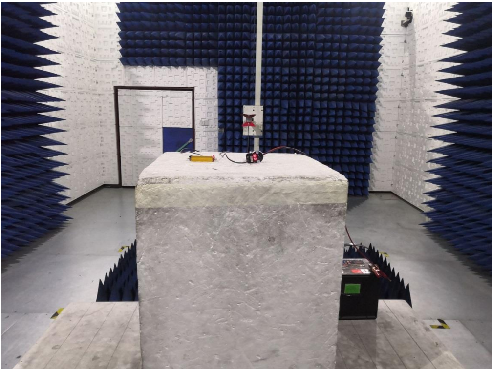
RADIATED EMISSION TEST SETUP ABOVE 1G
