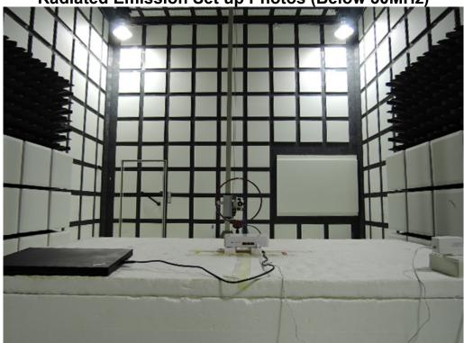
Radiated Emission Set up Photos (Below 1GHz)
