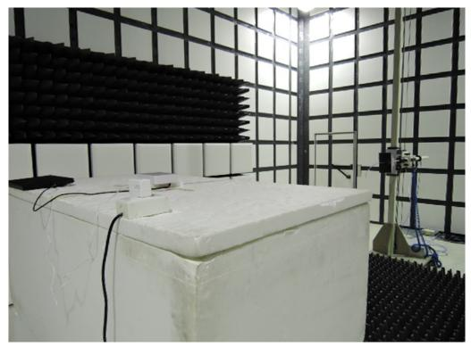
Radiated Emission Set up Photos (From View)
