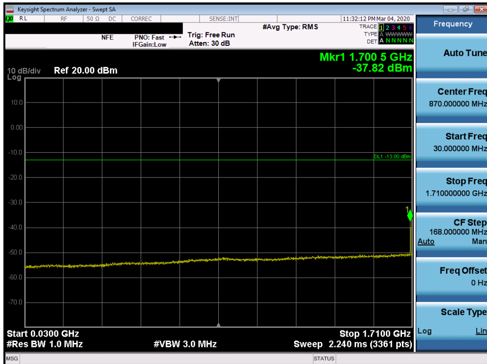
Plot 7-66. Conducted Spurious Plot (Band 66/4 - 20.0MHz QPSK - RB Size 1, RB Offset 0 - Mid Channel)
