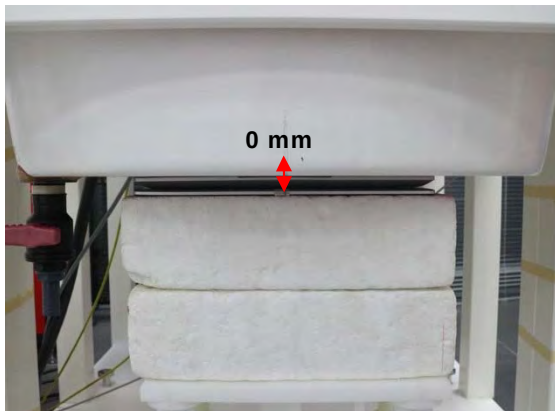
Fig.3 EUT Back side to flat phantom
