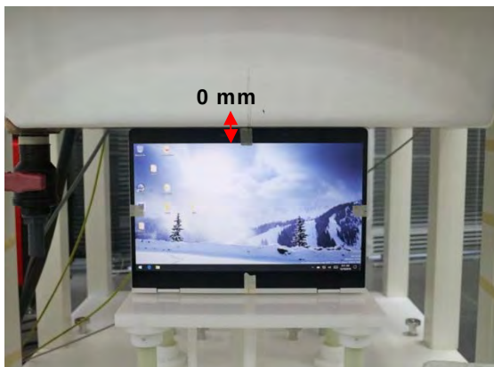
Fig.4 EUT Top side to flat phantom
