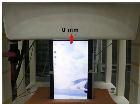
Fig.6 EUT Right side to flat phantom
