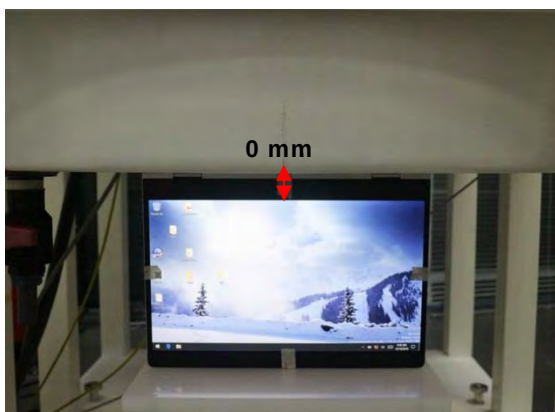
Fig.5 EUT Bottom side to flat phantom
