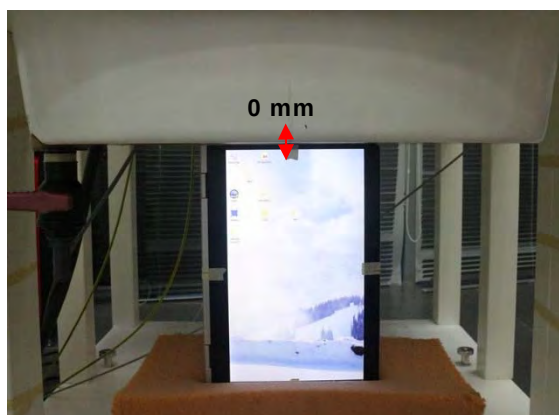
Fig.7 EUT Left side to flat phantom
