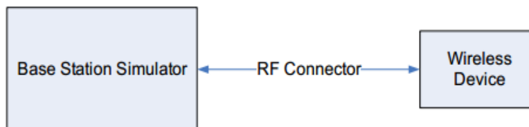
Figure 10.2 Power Measurement Setup
