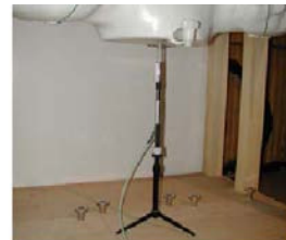
Figure 11.1 Dipole Verification Test Setup Diagram & Photo
