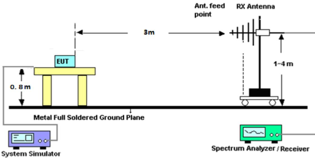
For radiated test from above 1GHz
