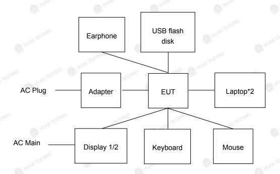
Operation of EUT during Radiation Above 1GHz testing:
