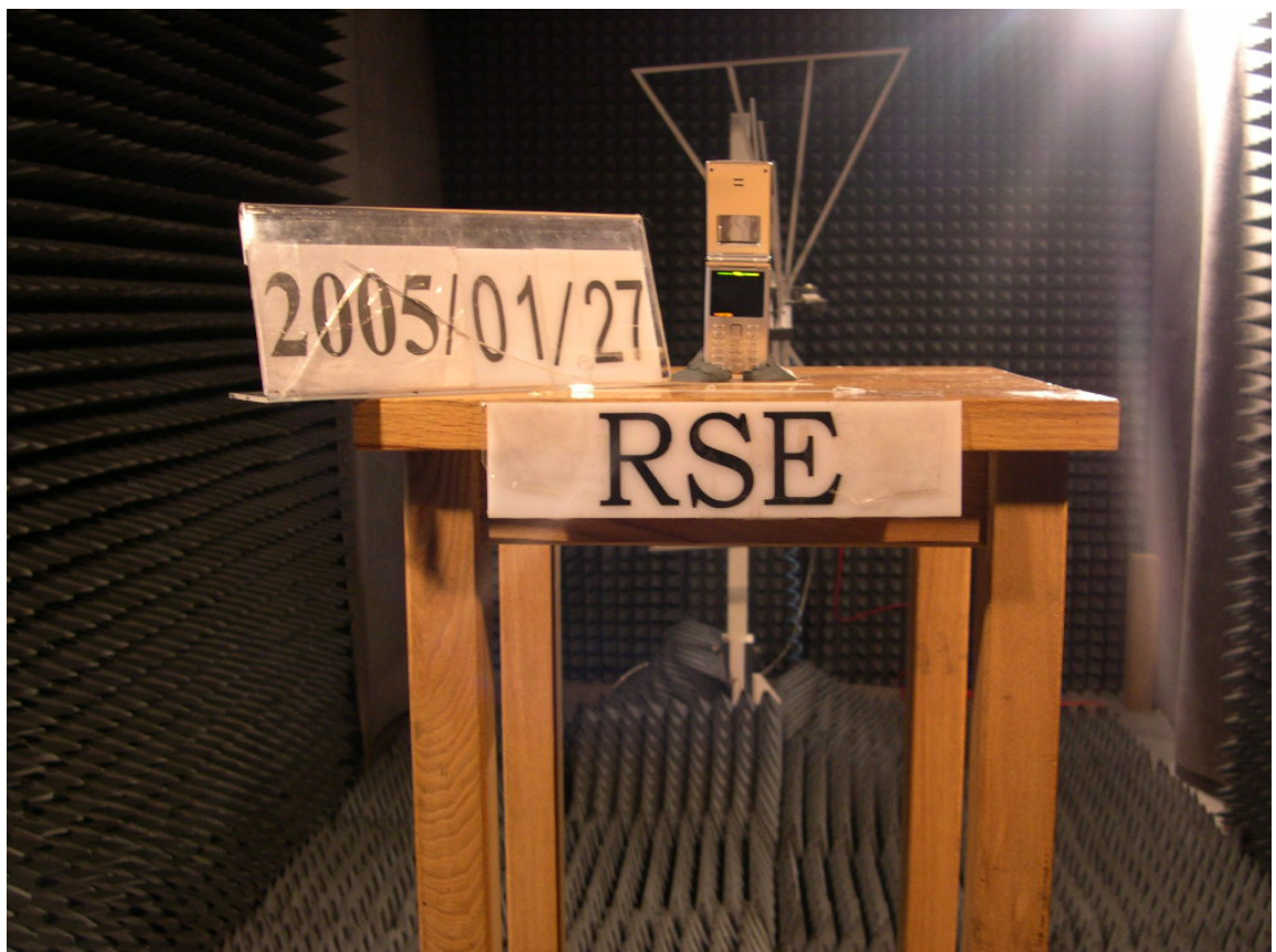
Pic2 Radiated Spurious Emission
