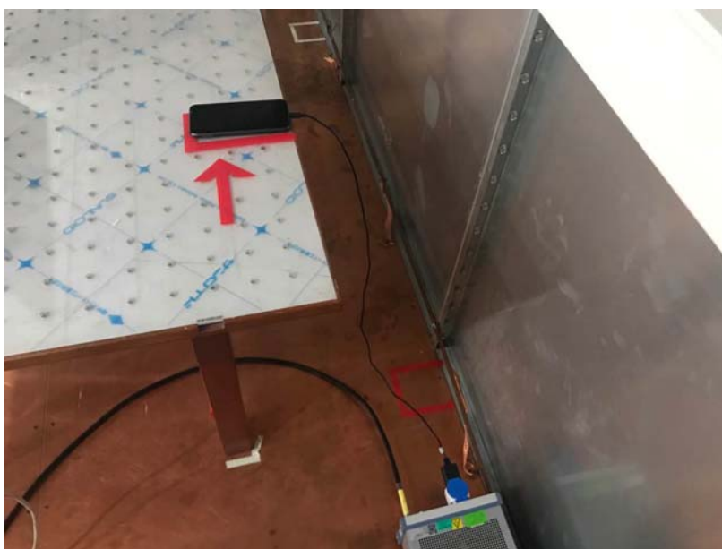
Conducted Emissions Test Setup (with charger)
