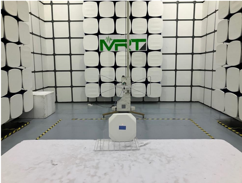
Description: Radiated Emission Test Setup for Above 1GHz Test Mode 2
