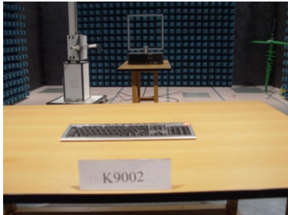
Photograph 1: Set-up for Radiation Measurement Below 30MHz
