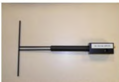
Figure 1 – Satimo COMOSAR Validation Dipole
