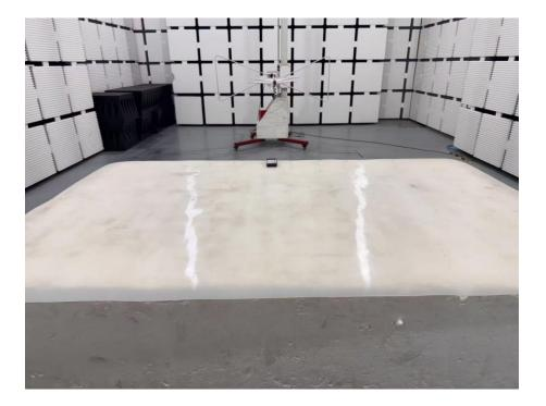
Set-up for Radiated Spurious Emission, Below 1GHz
