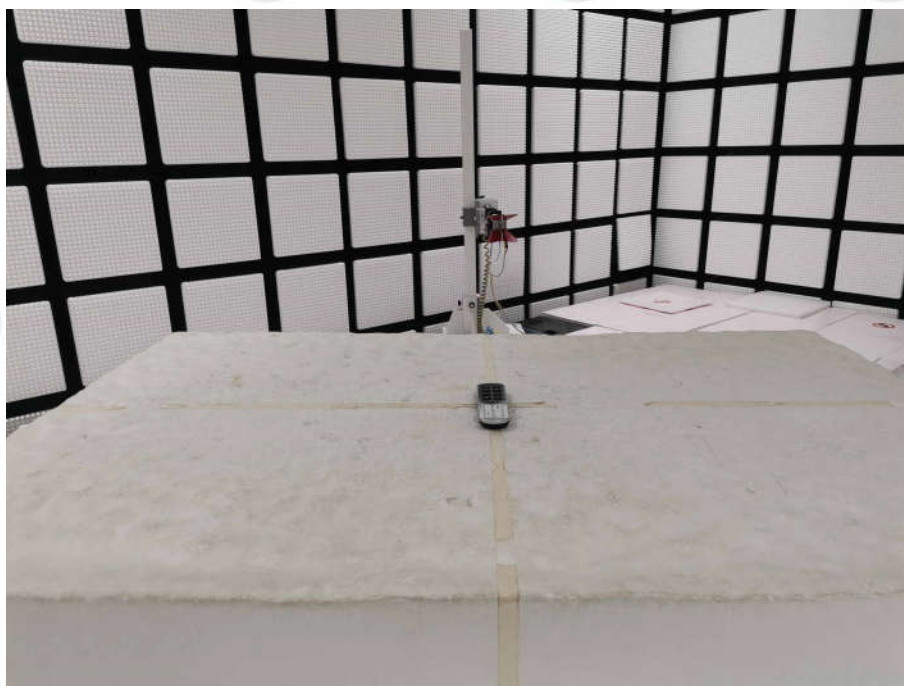
Radiated spurious emission Test Setup-2(Above 1GHz)
