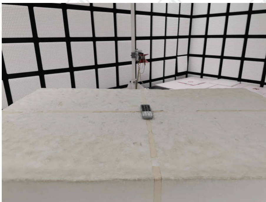
Radiated spurious emission Test Setup-2(Above 1GHz)
