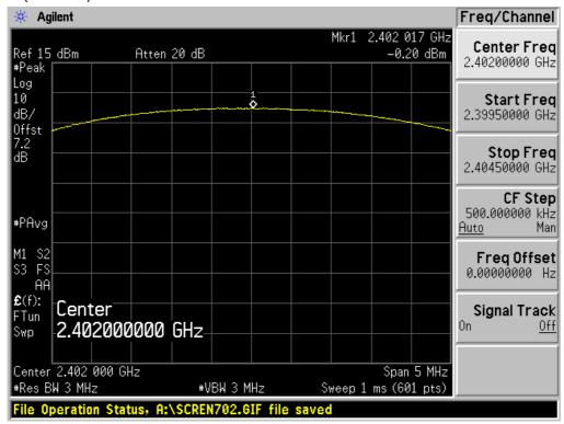
Test Plots (π/4DQPSK) Peak Power (Mid-CH)
