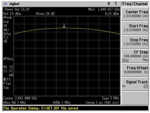
Test Plots (8DPSK) Peak Power (High-CH)
