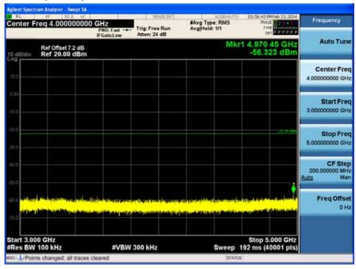
Test Plots (GFSK) - 5 GHz - 7 GHz Spurious Emission (Mid-CH)
