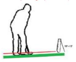
2) In outdoor or open areas (without a hitting net), if the detection capture rate is low, you can place the device and the ball at a  $10^{\circ}$  angle, which can improve radar wave detection (as shown in the diagram below).
