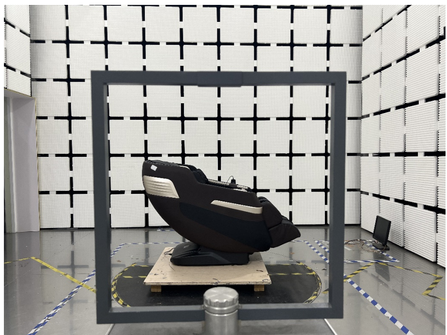
Radiation Emission Test Setup (Below 30MHz)
