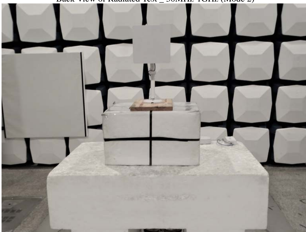
Back View of Radiated Test _ 30MHz-1GHz (Mode 2)
