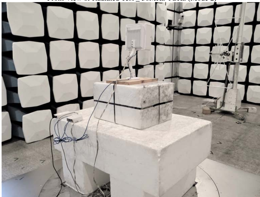
Front View of Radiated Test _ 30MHz-1GHz (Mode 2)
