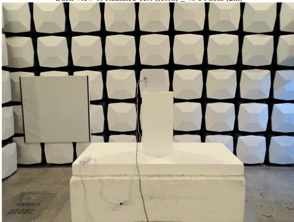
Back View of Radiated Test (Horn) _ 40-50GHz (2m)
