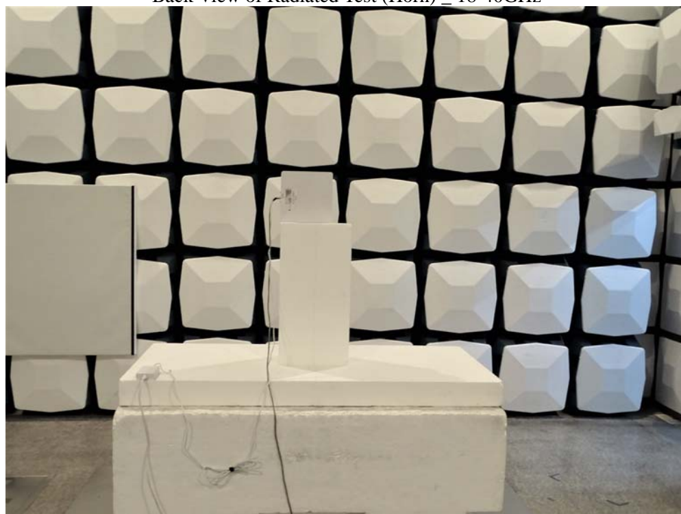
Back View of Radiated Test (Horn) _ 18-40GHz
