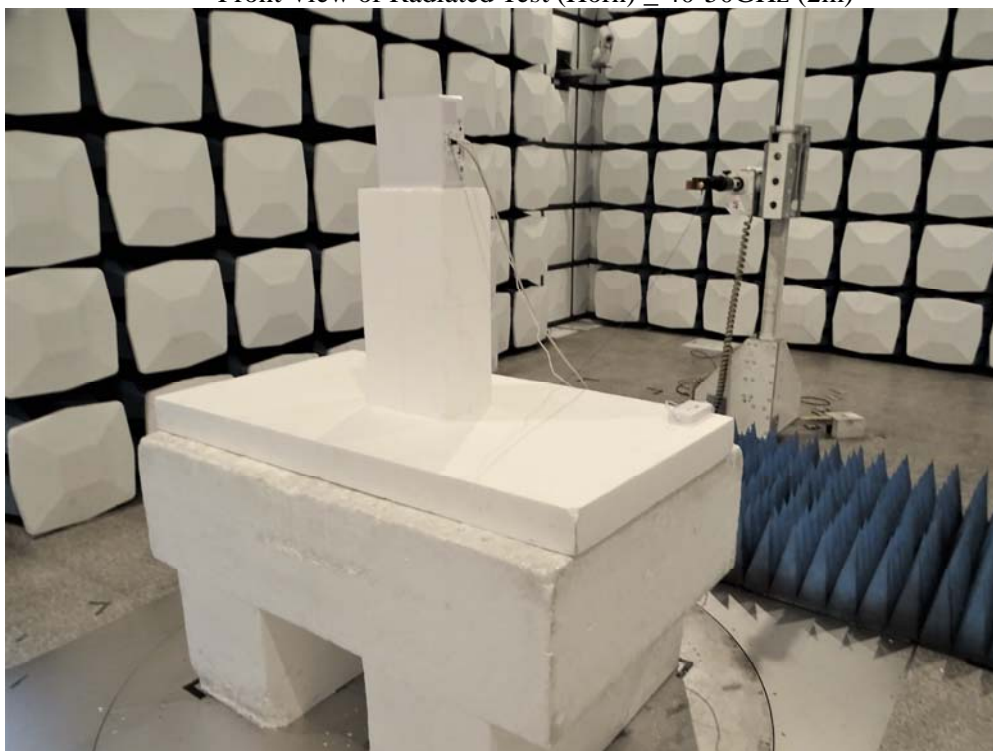
Front View of Radiated Test (Horn) _ 40-50GHz (2m)
