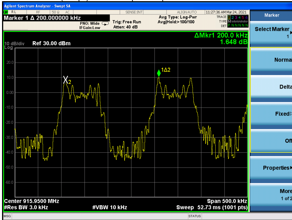
(1Mbps) Channel Separation plot on channel 102-103
