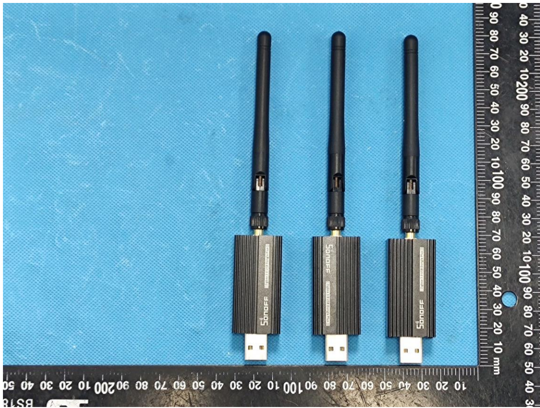
With Serial Chip: CP2102N-QFN28
