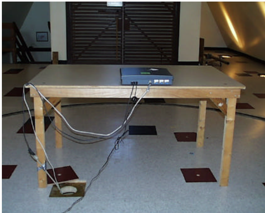
Photo 3 – Radiated Emissions Test Setup – Rear View
