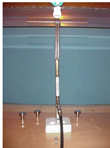
450 MHz Dipole Setup
