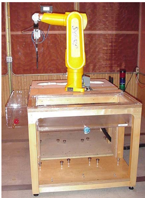
DASY4 SAR Measurement System with validation phantom
