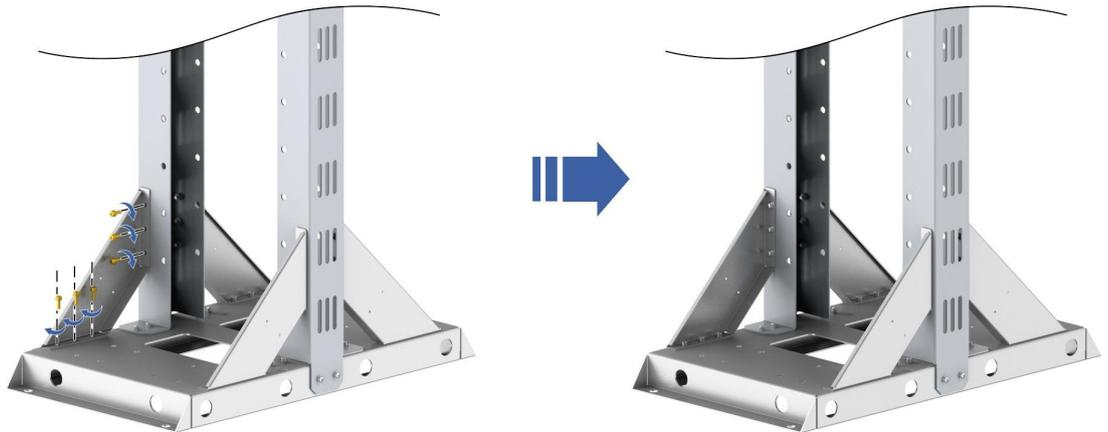
**Drilling Holes and Installing Expansion Bolts**
