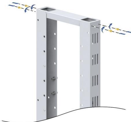
3. Install the two supporting plates with six M5 × 16 screws respectively, see [Figure 11-3](#).
