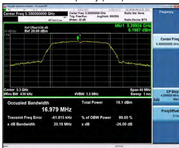
U-NII-2A, 802.11a Carrier frequency (MHz): 5300
