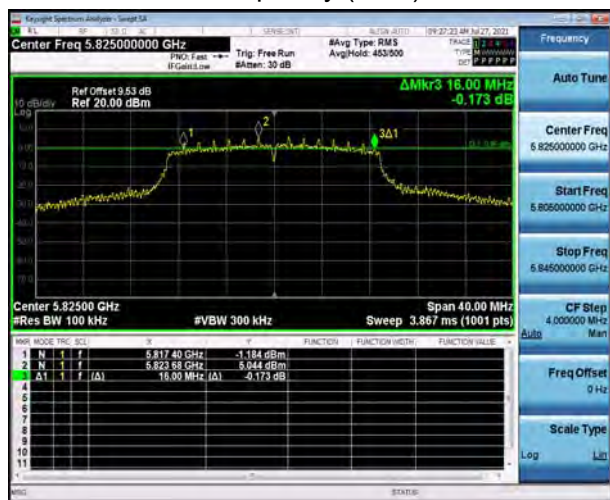
U-NII-3, 802.11ac VHT20 Carrier frequency (MHz): 5720
