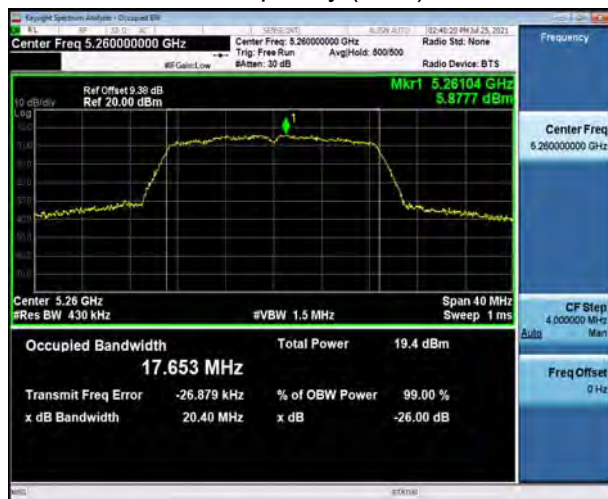
U-NII-2A, 802.11ac VHT20 Carrier frequency (MHz): 5300
