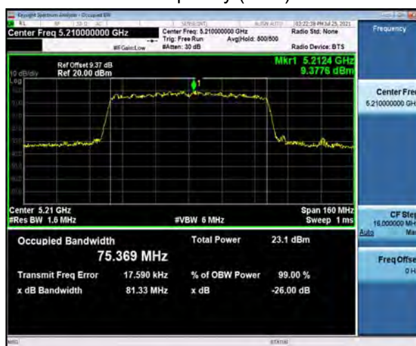
U-NII-2A, 802.11n HT20 Carrier frequency (MHz): 5260
