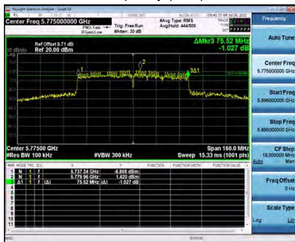
U-NII-3, 802.11ac VHT80 Carrier frequency (MHz): 5775
