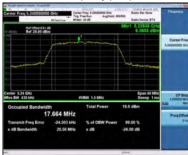
U-NII-1, 802.11ac VHT20 Carrier frequency (MHz): 5240
