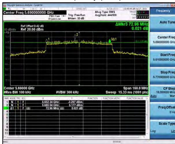
U-NII-3, 802.11ac VHT80 Carrier frequency (MHz): 5690
