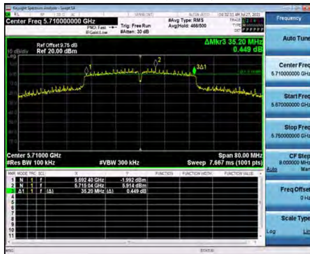
U-NII-3, 802.11ac VHT40 Carrier frequency (MHz): 5755
