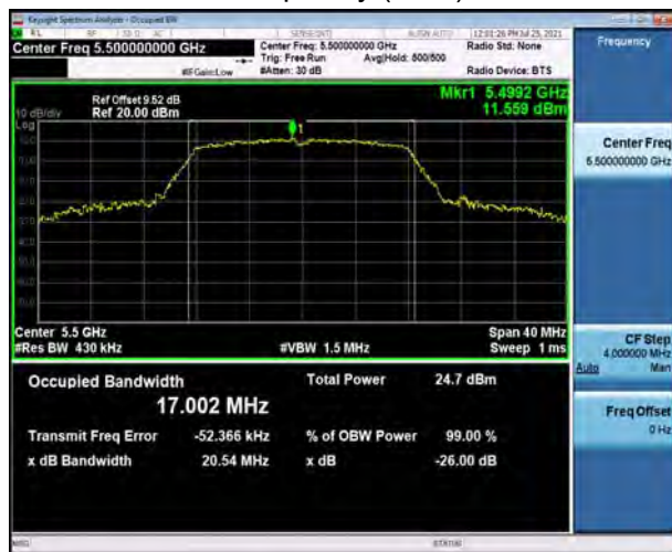
U-NII-2C, 802.11a Carrier frequency (MHz): 5500
