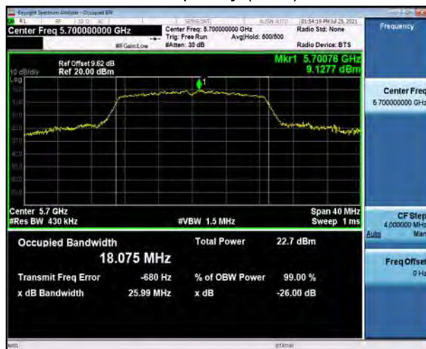
U-NII-2C, 802.11n HT20 Carrier frequency (MHz): 5720
