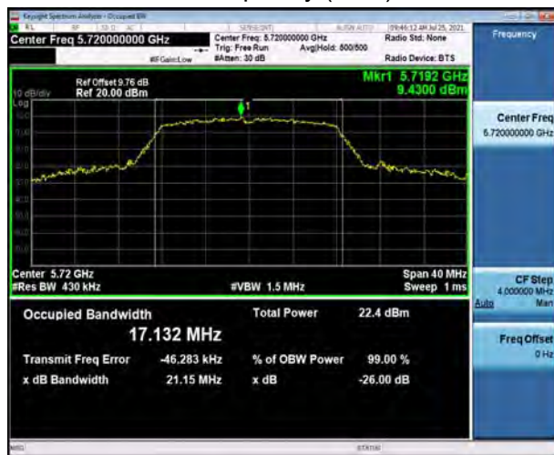
U-NII-2C, 802.11a Carrier frequency (MHz): 5720
