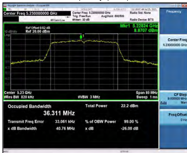
U-NII-1, 802.11ac VHT40 Carrier frequency (MHz): 5190
