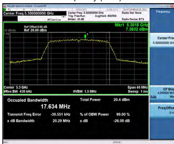
U-NII-2A, 802.11n HT20 Carrier frequency (MHz): 5300
