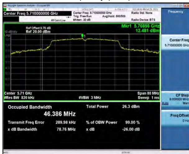
U-NII-3, 802.11n HT40 Carrier frequency (MHz): 5755
