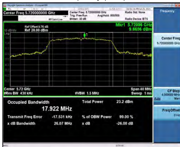
U-NII-3, 802.11ac VHT20 Carrier frequency (MHz): 5745
