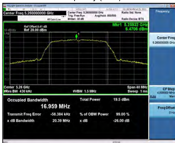
U-NII-2A, 802.11a Carrier frequency (MHz): 5300
