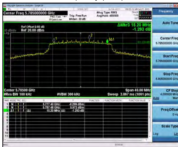
U-NII-3, 802.11ac VHT20 Carrier frequency (MHz): 5825
