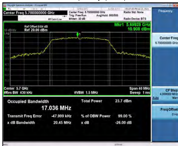
U-NII-2C, 802.11a Carrier frequency (MHz): 5720
