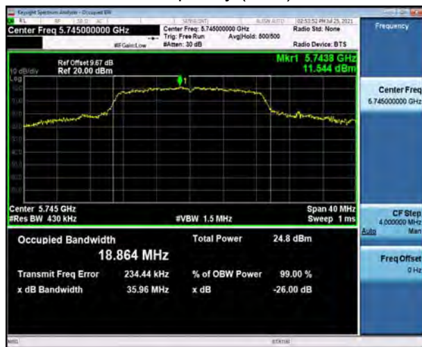
U-NII-3, 802.11ac VHT20 Carrier frequency (MHz): 5745
