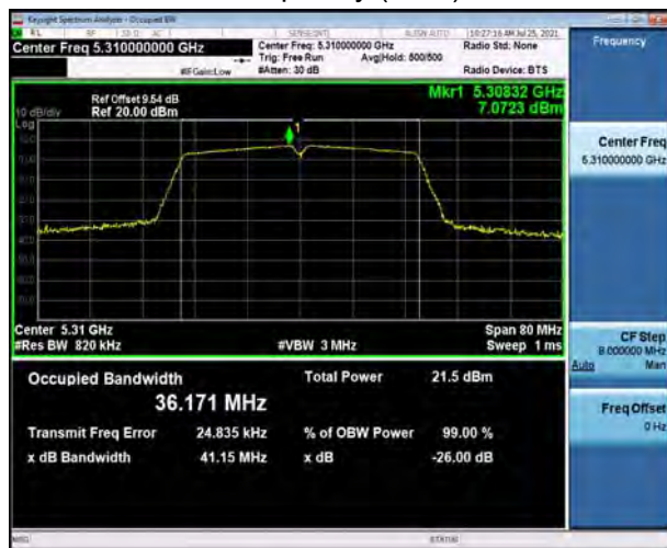
U-NII-2A, 802.11n HT40 Carrier frequency (MHz): 5310
