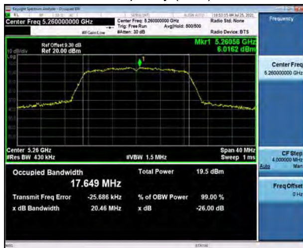
U-NII-2A, 802.11ac VHT20 Carrier frequency (MHz): 5300
