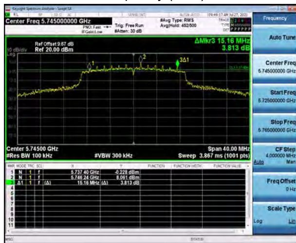
U-NII-3, 802.11ac VHT20 Carrier frequency (MHz): 5745
