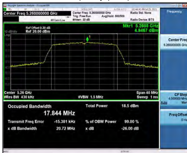
U-NII-2A, 802.11n HT20 Carrier frequency (MHz): 5300
