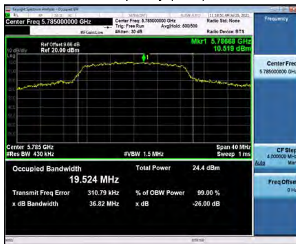
U-NII-3, 802.11ac VHT80 Carrier frequency (MHz): 5690
