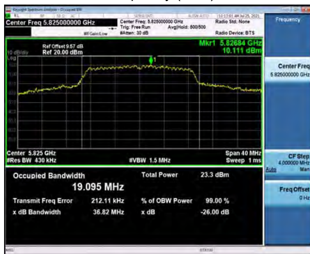
U-NII-3, 802.11ac VHT20 Carrier frequency (MHz): 5720
