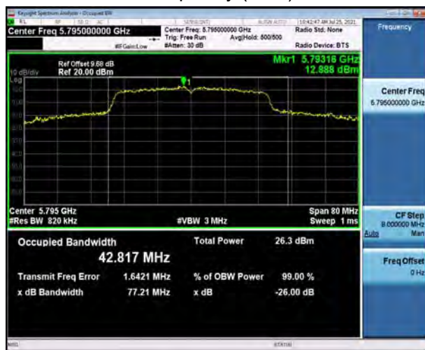
U-NII-3, 802.11ac VHT40 Carrier frequency (MHz): 5710
