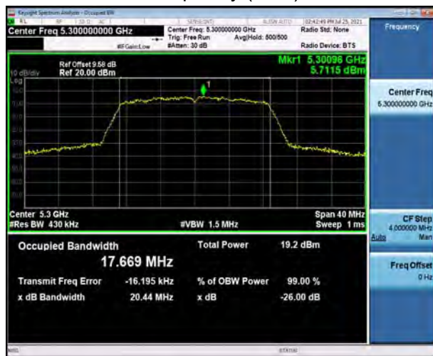
U-NII-2A, 802.11ac VHT20 Carrier frequency (MHz): 5300
