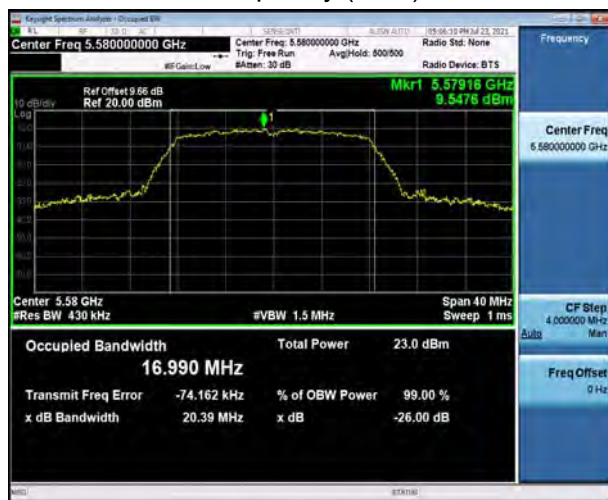
U-NII-2C, 802.11a Carrier frequency (MHz): 5700
