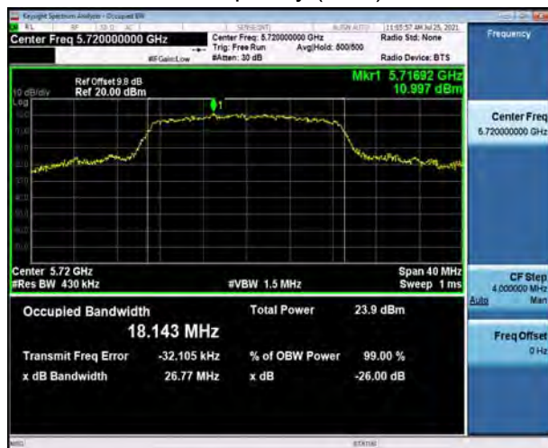
U-NII-3, 802.11ac VHT20 Carrier frequency (MHz): 5745
