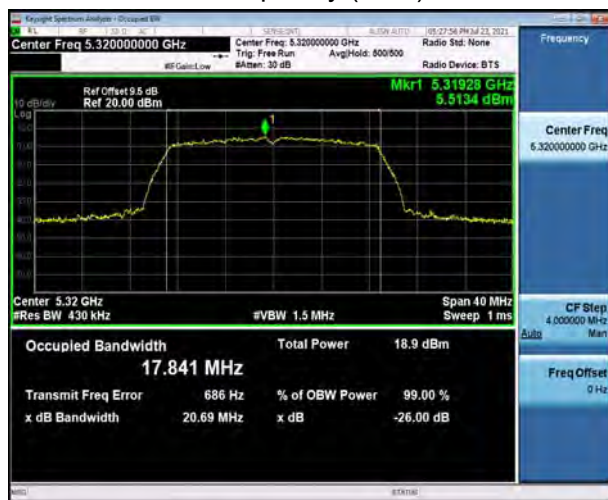
U-NII-2A, 802.11ac VHT20 Carrier frequency (MHz):5260
