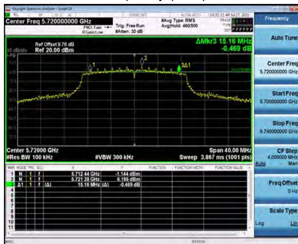
U-NII-3, 802.11ac VHT20 Carrier frequency (MHz): 5745
