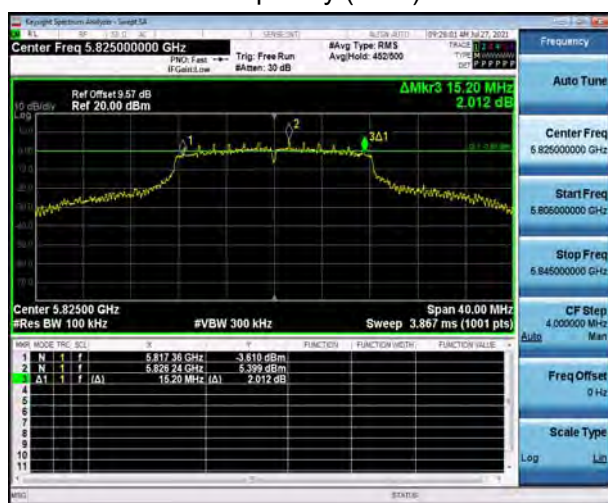
U-NII-3, 802.11n HT40 Carrier frequency (MHz): 5710
