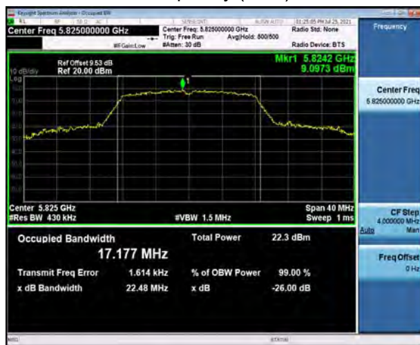
U-NII-3, 802.11n HT40 Carrier frequency (MHz): 5710
