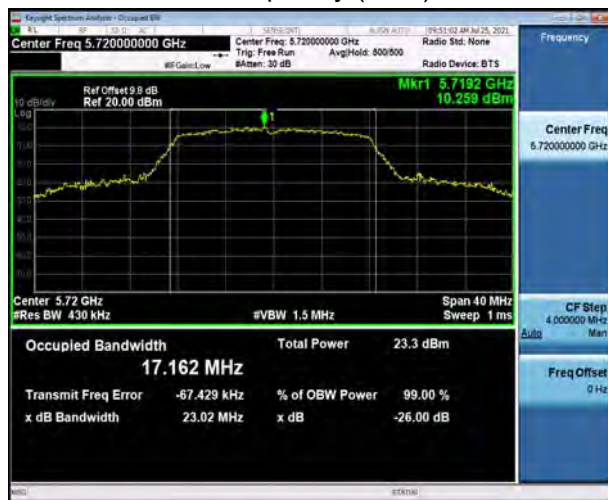
U-NII-2C, 802.11a Carrier frequency (MHz): 5720
