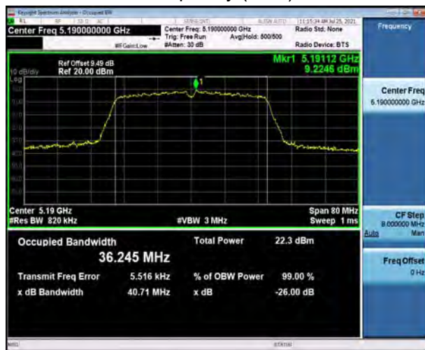
U-NII-1, 802.11ac VHT40 Carrier frequency (MHz): 5190
