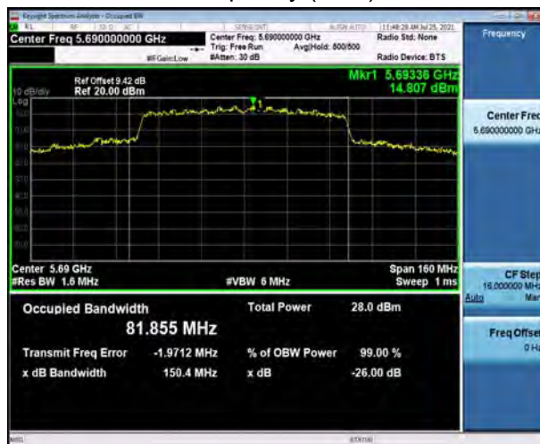
U-NII-3, 802.11ac VHT20 Carrier frequency (MHz): 5825
