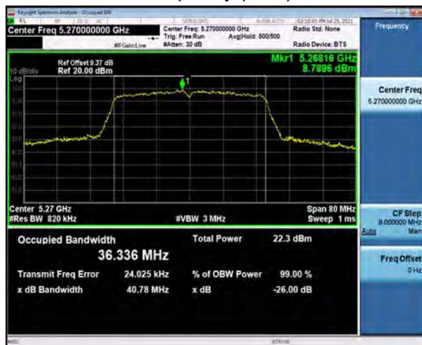
U-NII-2A, 802.11n HT40 Carrier frequency (MHz): 5310
