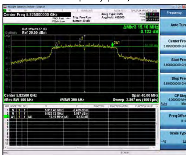
U-NII-3, 802.11ac VHT20 Carrier frequency (MHz): 5720
