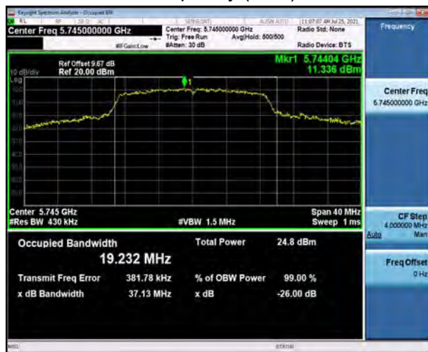
U-NII-3, 802.11ac VHT20 Carrier frequency (MHz): 5745
