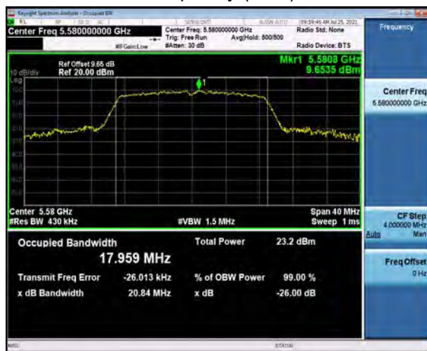
U-NII-2C, 802.11n HT20 Carrier frequency (MHz): 5700
