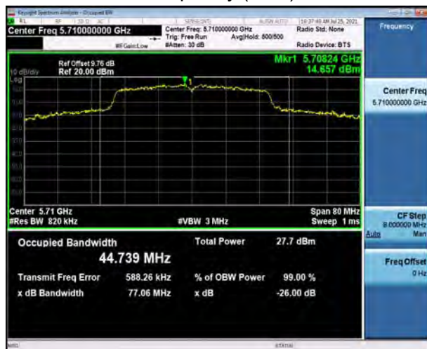
U-NII-3, 802.11n HT40 Carrier frequency (MHz): 5755
