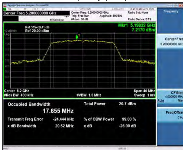
U-NII-1, 802.11ac VHT20 Carrier frequency (MHz): 5240
