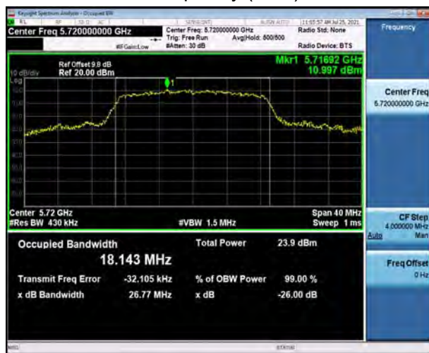
U-NII-2C, 802.11ac VHT80 Carrier frequency (MHz): 5530
