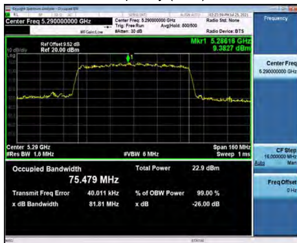
U-NII-2C, 802.11n HT20 Carrier frequency (MHz): 5500
