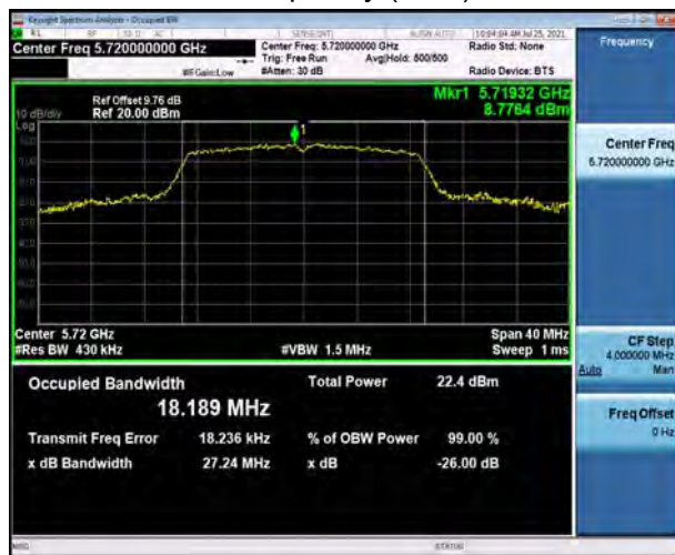
U-NII-2C, 802.11n HT20 Carrier frequency (MHz): 5720
