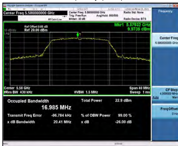
U-NII-2C, 802.11a Carrier frequency (MHz): 5700
