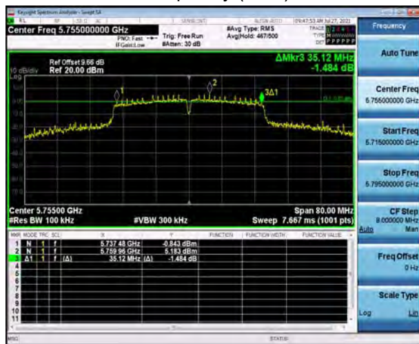
U-NII-3, 802.11n HT40 Carrier frequency (MHz): 5755
