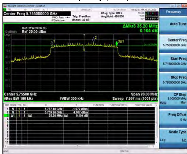
U-NII-3, 802.11ac VHT40 Carrier frequency (MHz): 5755
