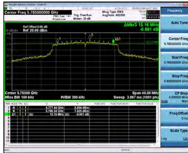
U-NII-3, 802.11ac VHT20 Carrier frequency (MHz): 5825
