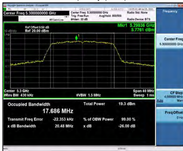
U-NII-2A, 802.11ac VHT20 Carrier frequency (MHz): 5300
