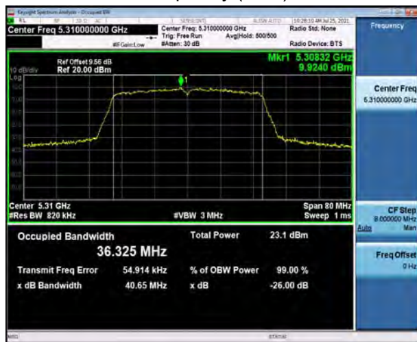
U-NII-2A, 802.11n HT40 Carrier frequency (MHz): 5310
