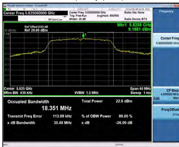
U-NII-3, 802.11ac VHT20 Carrier frequency (MHz): 5720
