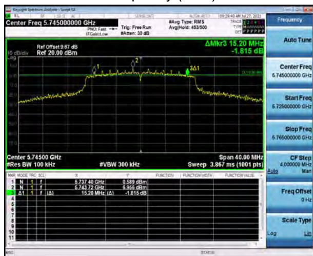
U-NII-3, 802.11ac VHT20 Carrier frequency (MHz): 5745
