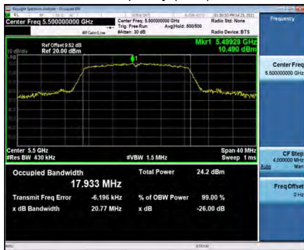
U-NII-2C, 802.11n HT20 Carrier frequency (MHz): 5500
