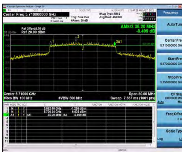
U-NII-3, 802.11n HT40 Carrier frequency (MHz): 5755
