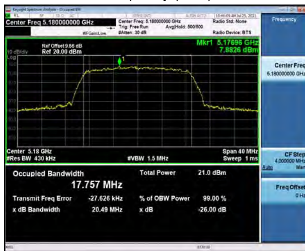
U-NII-1, 802.11ac VHT20 Carrier frequency (MHz): 5200
