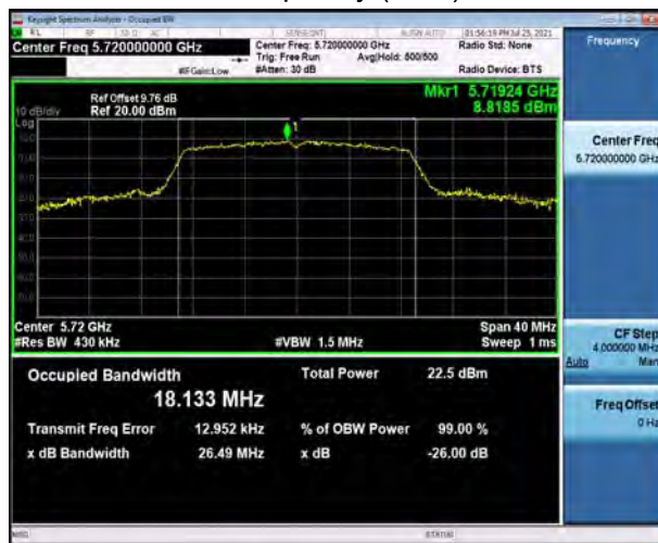
U-NII-2C, 802.11n HT20 Carrier frequency (MHz): 5720
