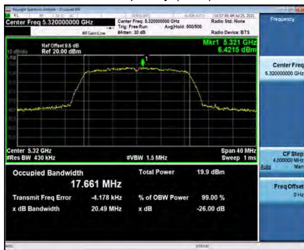
U-NII-2A, 802.11ac VHT80 Carrier frequency (MHz): 5290
