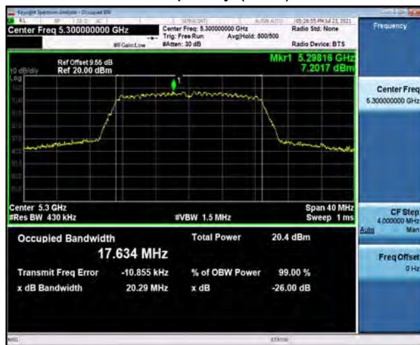
U-NII-2A, 802.11n HT20 Carrier frequency (MHz): 5300
