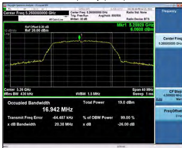
U-NII-2A, 802.11a Carrier frequency (MHz): 5300
