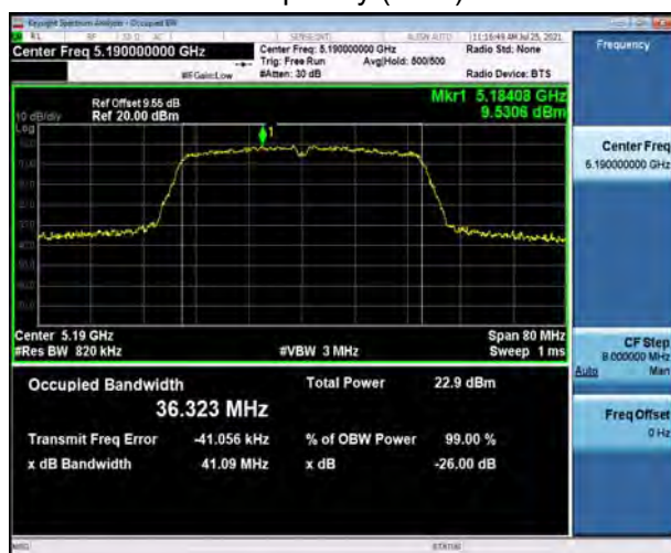
U-NII-1, 802.11ac VHT40 Carrier frequency (MHz): 5190
