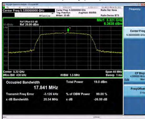
U-NII-2A, 802.11ac VHT20 Carrier frequency (MHz):5260
