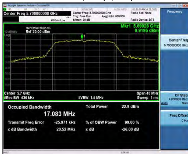
U-NII-2C, 802.11a Carrier frequency (MHz): 5720
