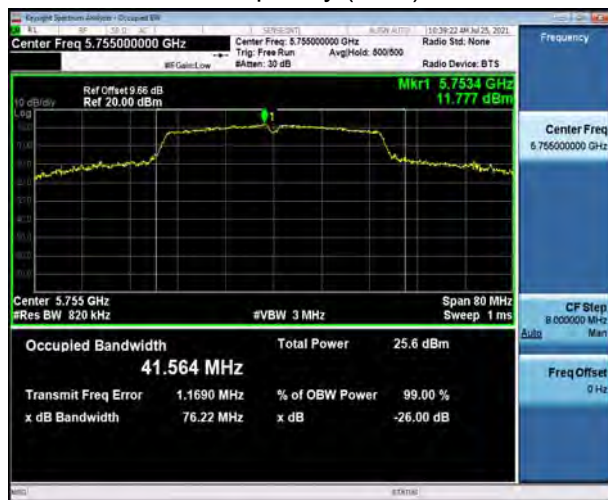
U-NII-3, 802.11n HT40 Carrier frequency (MHz): 5755
