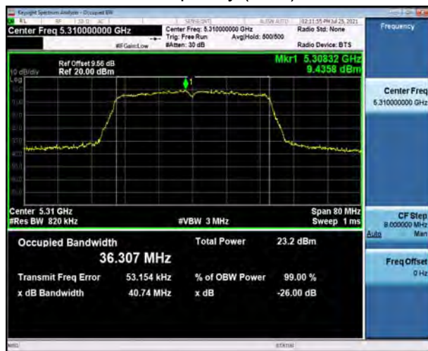
U-NII-2A, 802.11n HT40 Carrier frequency (MHz): 5310
