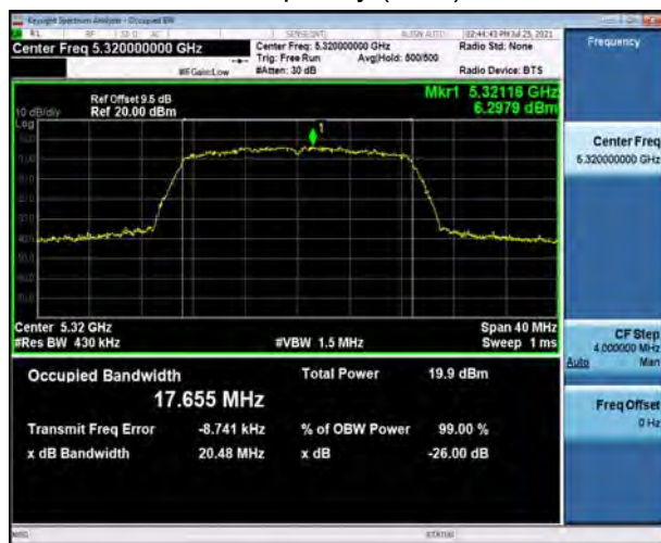
U-NII-2A, 802.11ac VHT80 Carrier frequency (MHz): 5290
