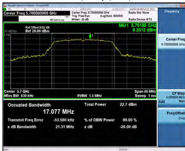
U-NII-2C, 802.11a Carrier frequency (MHz): 5720
