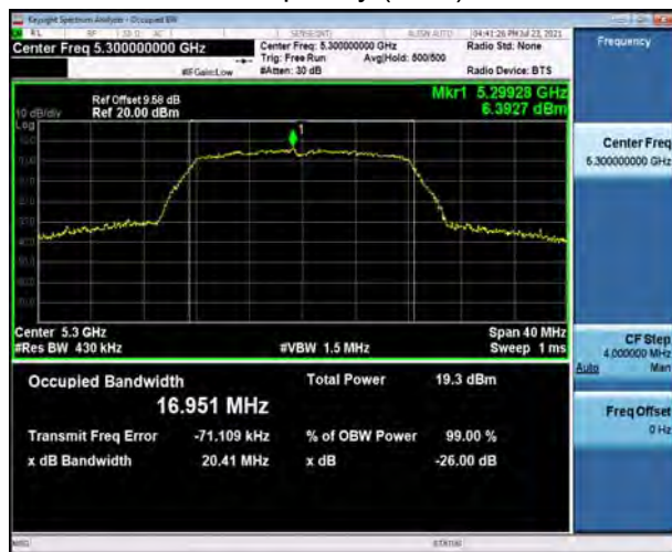
U-NII-2A, 802.11a Carrier frequency (MHz): 5300
