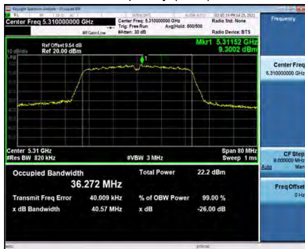
U-NII-2C, 802.11a Carrier frequency (MHz): 5500
