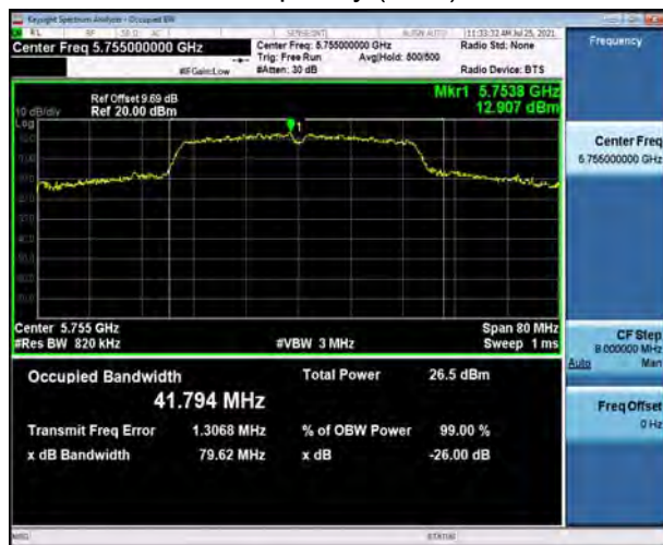
U-NII-3, 802.11ac VHT40 Carrier frequency (MHz): 5755
