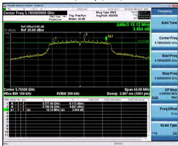
U-NII-3, 802.11ac VHT20 Carrier frequency (MHz): 5825
