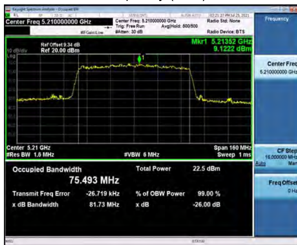
U-NII-2A, 802.11n HT20 Carrier frequency (MHz): 5260
