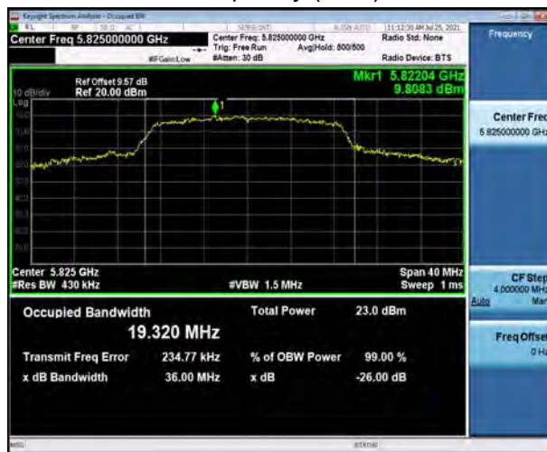
U-NII-3, 802.11ac VHT20 Carrier frequency (MHz): 5825
