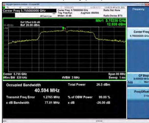
U-NII-3, 802.11n HT40 Carrier frequency (MHz): 5755
