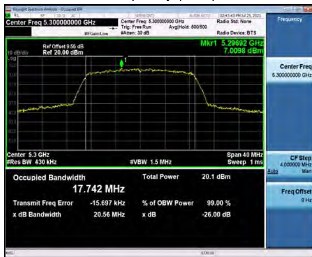
U-NII-2A, 802.11ac VHT20 Carrier frequency (MHz): 5300
