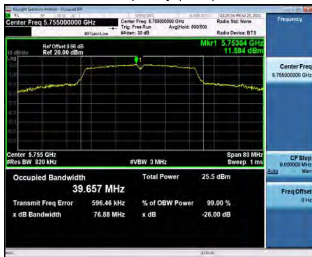
U-NII-3, 802.11n HT40 Carrier frequency (MHz): 5755
