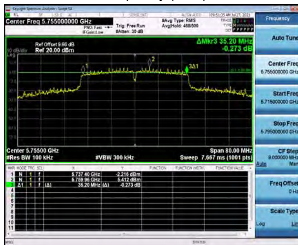
U-NII-3, 802.11ac VHT40 Carrier frequency (MHz): 5755
