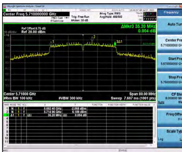
U-NII-3, 802.11n HT40 Carrier frequency (MHz): 5755
