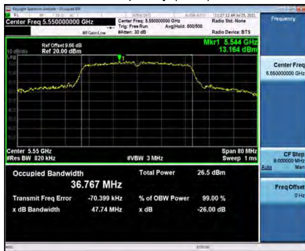
U-NII-2C, 802.11ac VHT40 Carrier frequency (MHz): 5550
