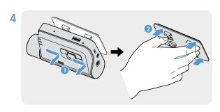
Remove the product from the mount and push the mount against the windshield to ensure that the mount is firmly fixed.
