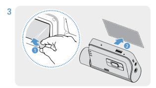
Remove the protective film from the adhesive mount, and then press the mount to the installation location.
