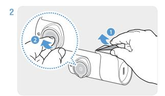
Remove the protective film from the adhesive mount and camera lens.
