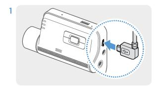
Connect one end of the rear camera cable to the front camera's V-IN port.
