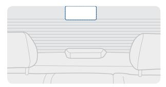
Select a location on the rear windshield where there is no defrost grid wire and the camera can record the entire rear view.
