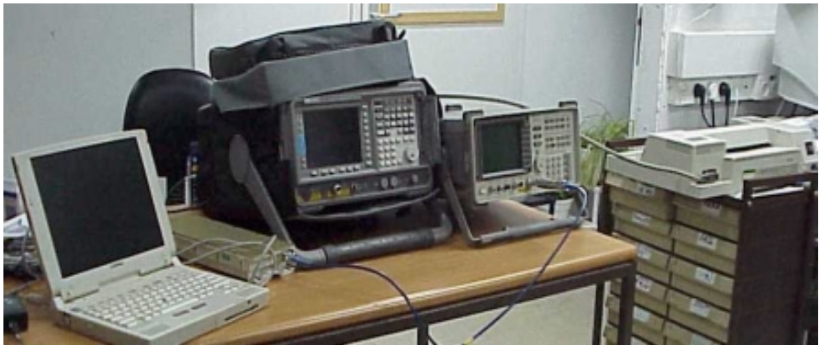
Photo #10 Spurious conducted antenna test. Measuring equipment
