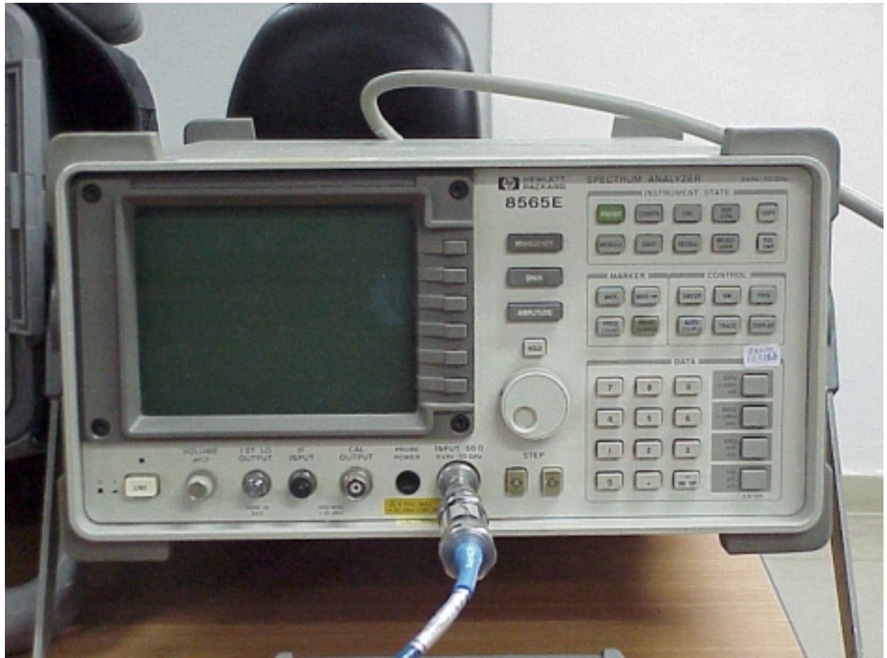
Photo #11 Spurious conducted antenna test. Measuring equipment
